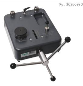
In addition the series LR-Cal LSP-H feature a threaded spindle which only runs within the pump body. Thus there is no adverse bending moment acting on an outstanding spindle, and particularly for field use this has the advantage that the dimension of these pressure comparison pumps will not change when the spindle is turned during operation. The series LR-Cal LSP-H needs only little force to generate also high pressures.
