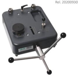
In addition the series LR-Cal LSP-H feature a threaded spindle which only runs within the pump body. Thus there is no adverse bending moment acting on an outstanding spindle, and particularly for field use this has the advantage that the dimension of these pressure comparison pumps will not change when the spindle is turned during operation. The series LR-Cal LSP-H needs only little force to generate also high pressures.
