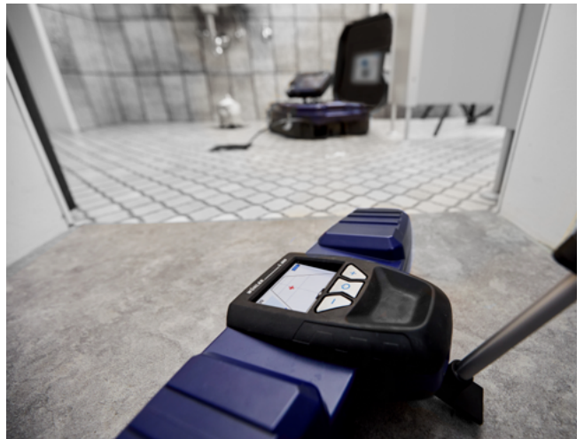
Precise location of the camera head with the Wöhler L 200 Locator.
