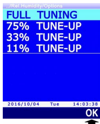
Fig. 13.3.4: types of RH sensor calibration
