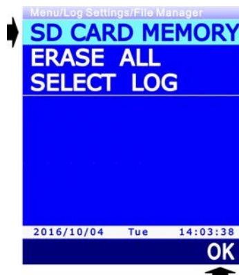
Fig. 7.11.1: selecting the SD CARD MEMORY menu item
