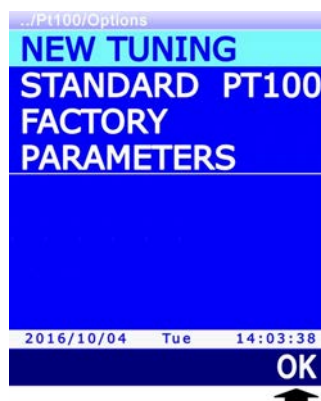
Fig. 13.2.1: PRT probe calibration types
