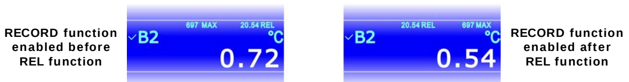
Fig. 5.6.1: activation order of RECORD and REL functions
