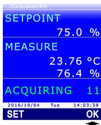
Fig. 13.3.6: calibration point confirmation
