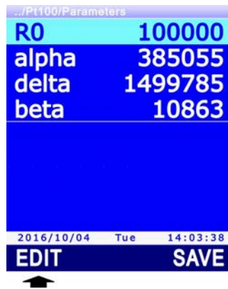
Fig. 13.2.3: parameters for temperature calculation equation
