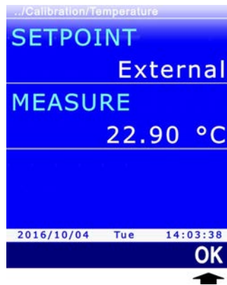
Fig. 13.3.3: calibration of the Pt100 sensor to the reference value
