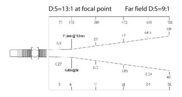
D:S is the optical resolution expressed as a ratio of the distance to the target spot divided by the diameter of the spot.
