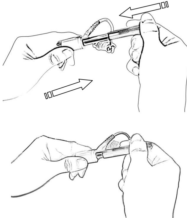
Hold the impact device with left hand while push the loading tube with right hand toward to the end. Then loose the force and let the loading tube back to original position.
