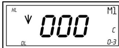
Take 3 measurements (impact direction: downward
