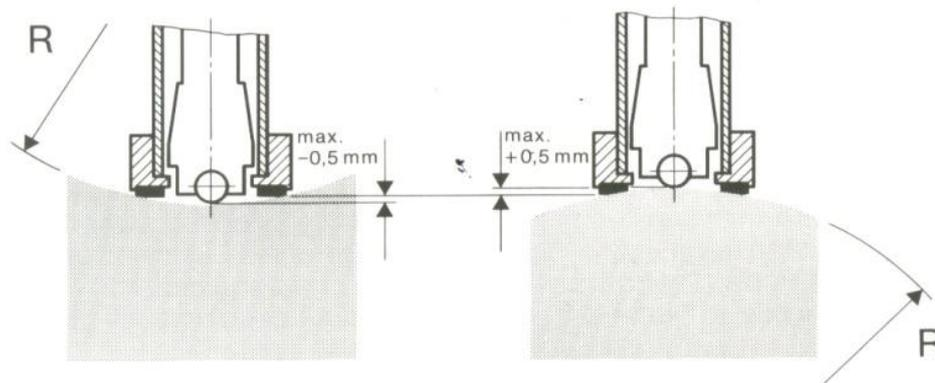
Impact device types D, D+15 and C  $R_{min} = 30mm$
