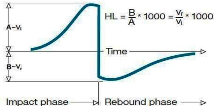
Voltage characteristic of output signal
