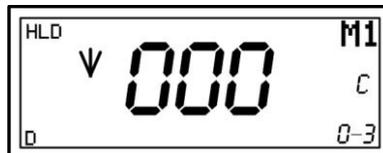
At the mode of calibration, you are asked to take 3 measurements (impact direction: downward ↓) on standard test block in total. Please follow up the direction indication on LCD to take measurements.
