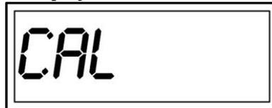
Press and hold Key
