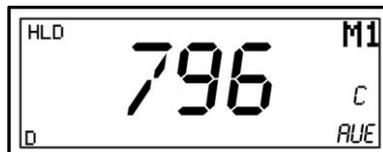
If the average value differs from the standard value of test block, you can press and hold key
