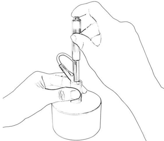
Place the impact device against the object to be measured. Then press the release button on top of the impact device with finger of right hand. The measuring value will display on LCD.
